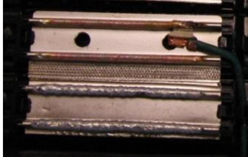
Figure 25 – Two types of bus bars ultrasonically bonded in the center to each other
