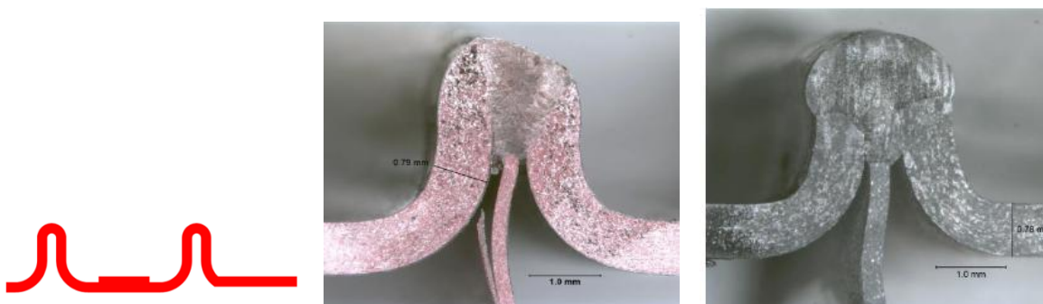
Figure 24 – Bus bar concept diagram and resulting welded cross sections
