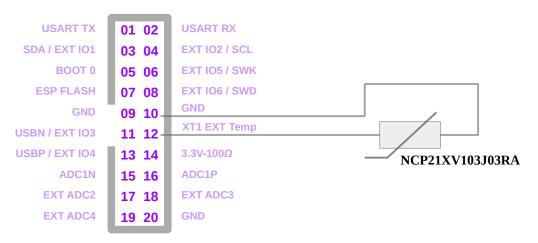
The SBMS is calibrated for a particular  $10k\Omega$  thermistor made by Murata NCP21XV103J03RA (this same thermistor type is used internally to measure the power board temperature).
