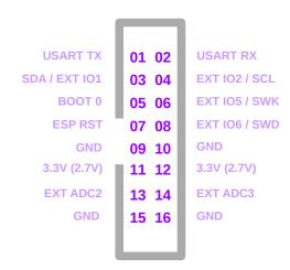
01 & 02 UART TX and RX pins are used for the WiFi module so if you want to use the USART for something else then WiFi will be disabled (voltage levels 0 to 3.3V).
