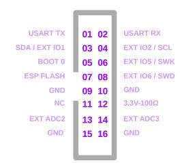
01 & 02 UART TX and RX pins are used for the WiFi module so if you want to use the USART for something else then WiFi will be disabled (voltage levels 0 to 3.3V).
