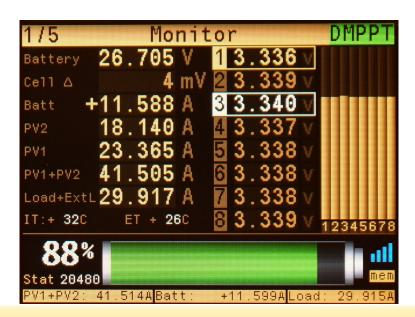
By pressing the OK button while in this menu you will be presented with a small submenu allowing you to change the display from current measured with 1mA resolution to power measured with a 0.1W resolution and also allowing you to change the temperature units from Celsius to Fahrenheit
