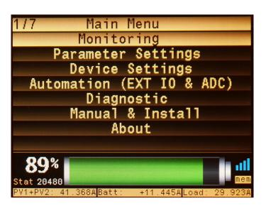
\* SOC (State Of Charge) indication will be set automatically to 50% (49%) when you connect the SBMS to battery for the first time since SBMS can not guess the state of charge based only on cell voltage.
