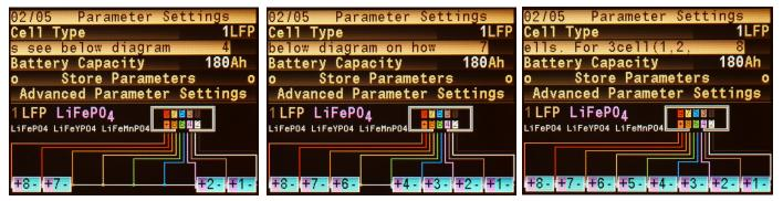
\*Screenshots for SBMS40 the SBMS0 has a 12pin cell balancing connector so diagram will look different. Photo from SBMS0 will be updated in next revision of the user manual.
